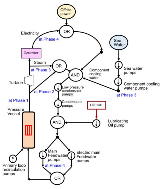
Fig. 2. Topological relation of a BWR plant system.
